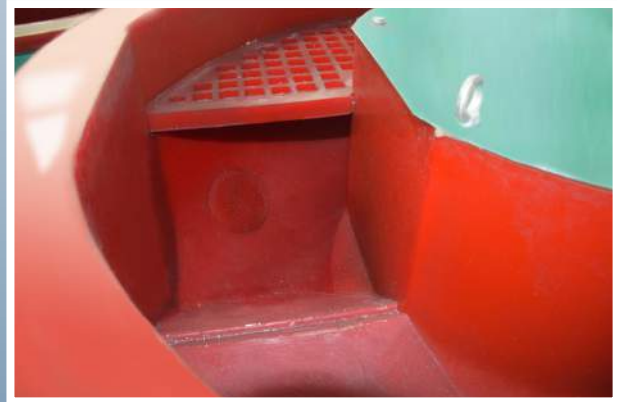
CL- AB type: spiral curved mouth with automatic separation sieve
