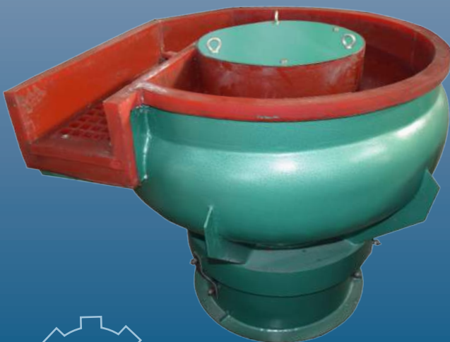
CL- AB type: spiral curved mouth with automatic separation sieve
